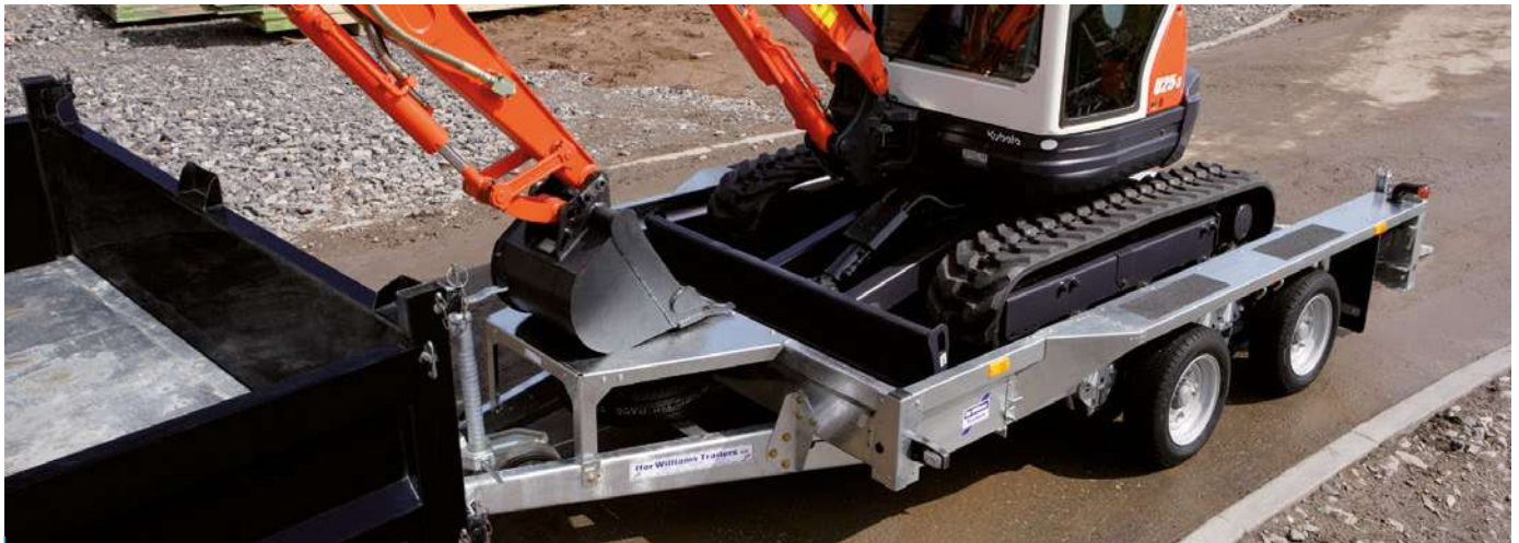
GX106 with skids and integrated rear supports
