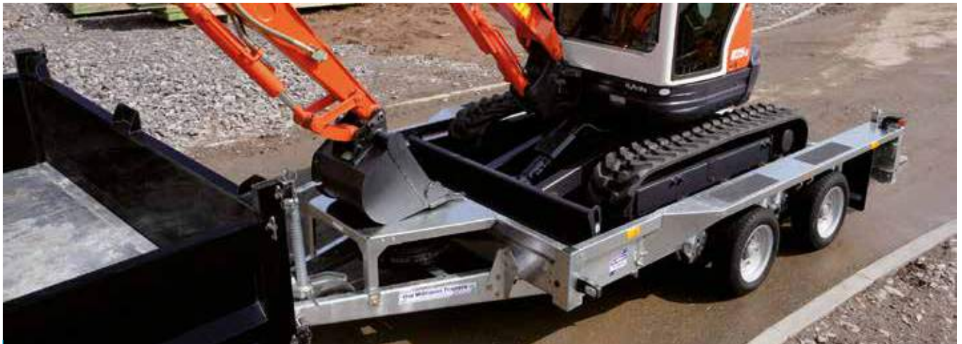
GX106 with skids and integrated rear supports
