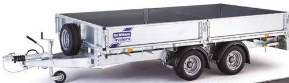
LM126 with optional dropsides, tailboard and headboard.
