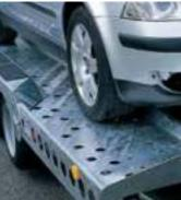
**Perforated Platform** The whole of the trailer platform is perforated to provide both traction and multiple lashing positions.
