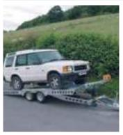
**Uncoupled Loading** A special skid under the coupling allows the trailer to be loaded when uncoupled. This avoids overloading the towing vehicle towball when loading heavier vehicles.
