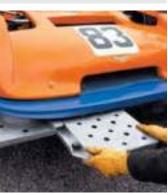
Skids do not protrude beyond the trailer deck, and can be refitted beneath the lowest of vehicles.
