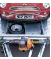
**Fitted Spare Wheel and Lockable Toolbox** Concealed neatly below the deck level, both are included as standard (optional GM5 winch shown).
