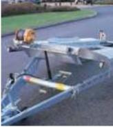
**Galvanized Construction** and Hydraulic Tilt System Galvanized steel deck and drawbar constructed from high tensile steel for maximum strength to weight ratio.
