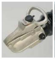
**Coupling Head** The lockable low-profile coupling head ensures optimum clearance of 4x4 rear doors (also standard on CT136HD).
