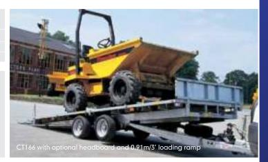
CT166 with optional 0.91m/3' loading ramp (0.3m/1' loading ramp comes as standard)
