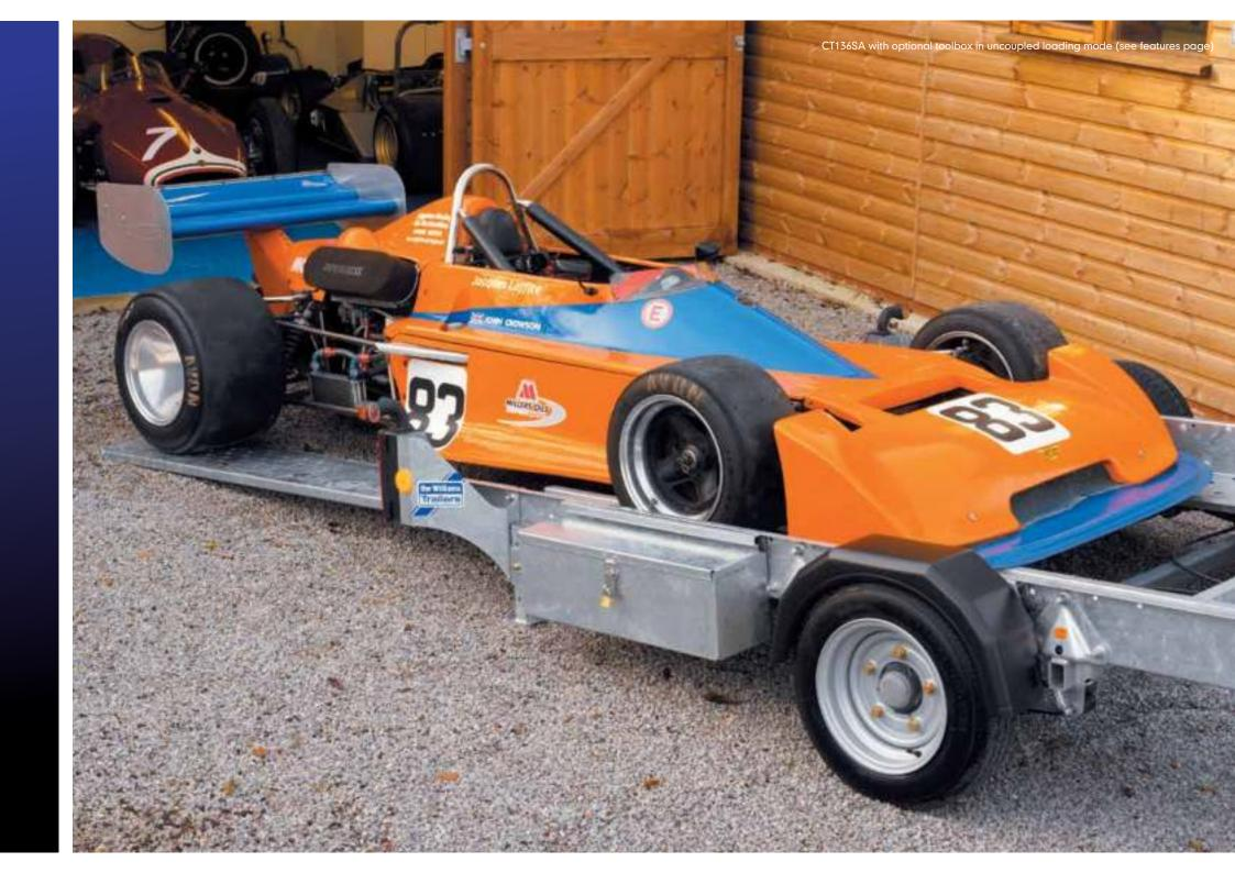
CT136SA single axle with spare wheel and wheel chocks
