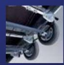
**Chassis** The underside of the trailer features a galvanized steel chassis and drawbar, for longlasting corrosion protection.
