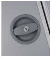
Lockable Grooms Door Flush fitting locking mechanism, provides privacy for riders if used for changing at a show. Grooms doors can be positioned on either side of the trailer.
