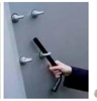
**Breast Bar Release System** Enables the release of breast bars safely from outside of the trailer. Conveniently suits the wheel brace supplied with each horsebox.
