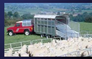
EasyLoad™ deployed and rear barrier lowered.
