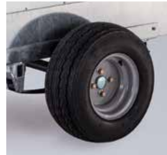
Q5/6/7e off-road flotation tyres (20.5 x 8-10)
