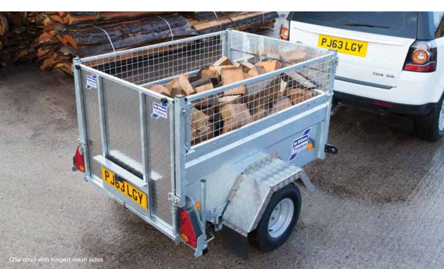
Q5 Q5e off-road and road versions showing different ramp, hinged sides and internal partition options
