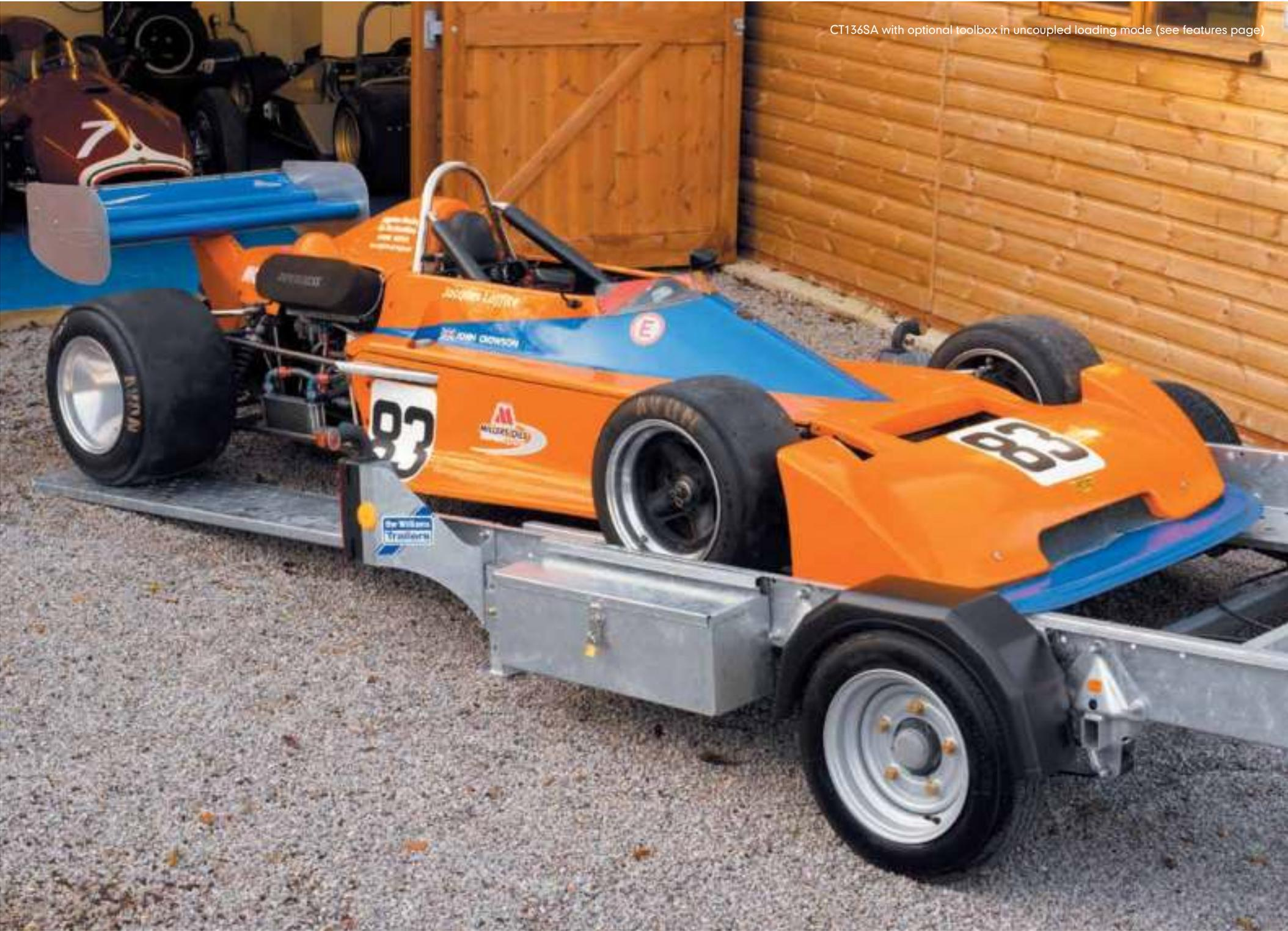
**CT136SA** single axle with spare wheel and wheel chocks
