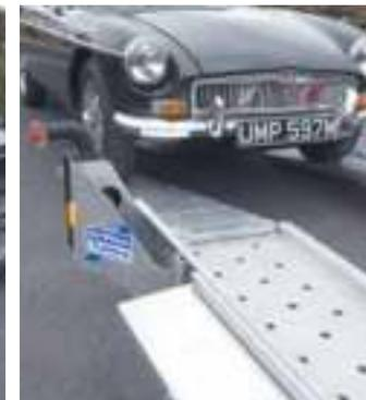
Lights are positioned well clear of the trailer body.
