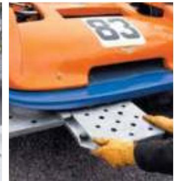
Skids do not protrude beyond the trailer deck, and can be refitted beneath the lowest of vehicles.
