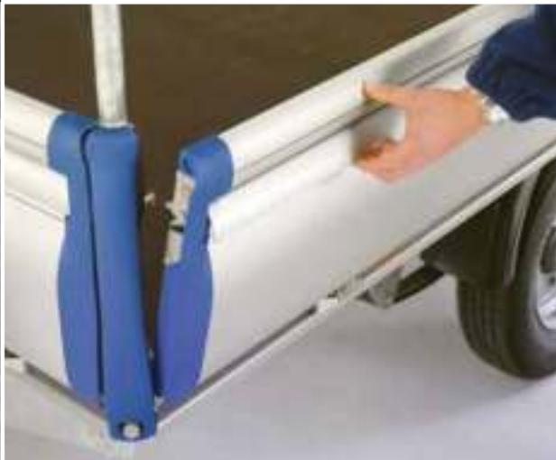
To release the Aluminium dropsides simply apply slight inward pressure to the dropside then lift the latch with fingers to release. The dropsides will only release when pressed inwards prior to the latch being lifted (Lifting the latch alone will not release the dropside).
