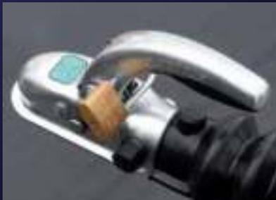
The lockable coupling head can be locked on or off the tow ball for additional security (Padlock not included).
