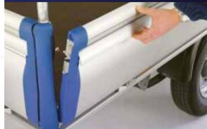
To release the Aluminium dropsides simply apply slight inward pressure to the dropside then lift the latch with fingers to release. The dropsides will only release when pressed inwards prior to the latch being lifted (Lifting the latch alone will not release the dropside).
