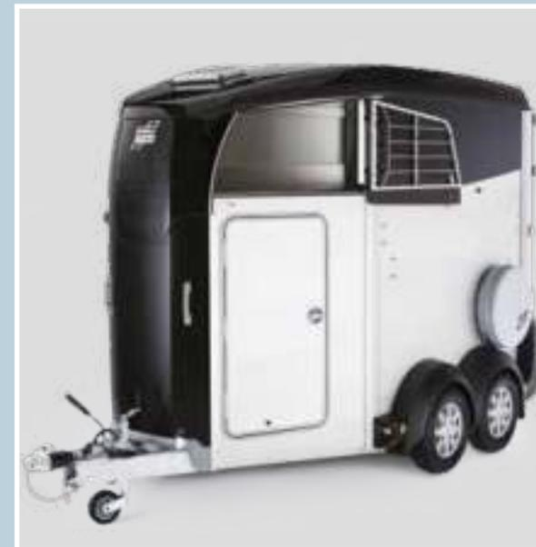
When ordering your **HBX**, you can choose either a left-hand ramp, a right-hand ramp or a built-in tack locker, the inspection door is fitted to the opposite side. A front ramp is not available if the tack locker is installed. There is no front ramp on the **HBE**.
