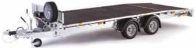
LM166B with optional electric winch (and battery) and optional propstands
