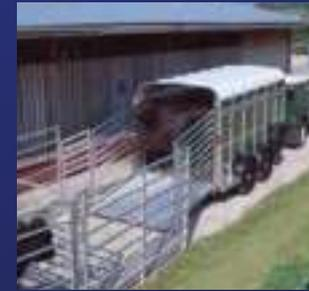
The TA5 6' headroom is available in 8', 10', 12' and **now** 14' body lengths. The 7' is available in 10', 12' and **now** 14' lengths. The 8' and 10' versions have a maximum gross weight of 2700kg, while the 12', 14' and heavy duty version offers 3500kg maximum gross weight.
