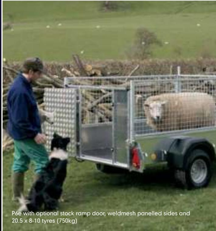
P6e with optional stock ramp door, weldmesh panelled sides and 20.5 x 8-10 tyres (750kg)
