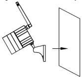
Camera can be attached by strong magnetic base or Gopro compatible holder
